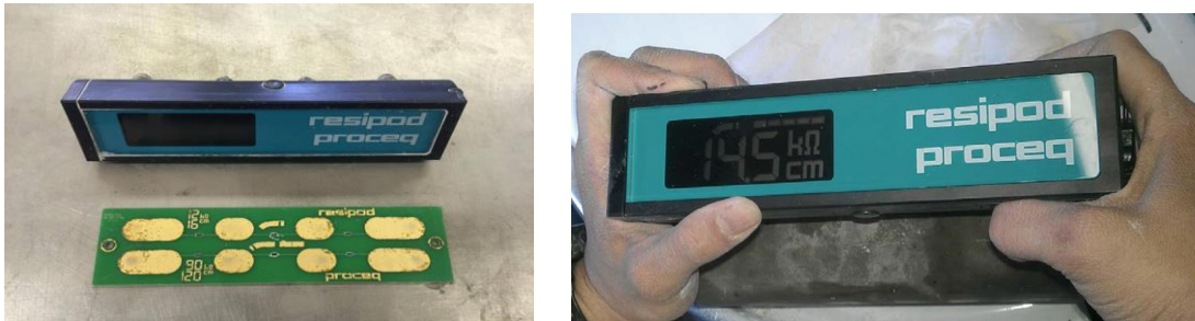
Figure 1. Measuring Surface Electrical Resistivity with 4-Point Wenner Probe
