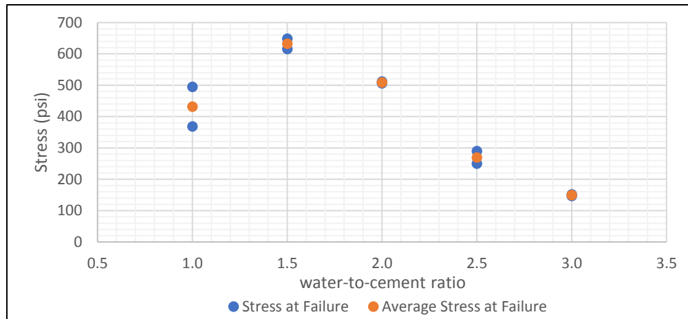
Figure 2: 28-day water-to-cement ratio vs. stress at failure
