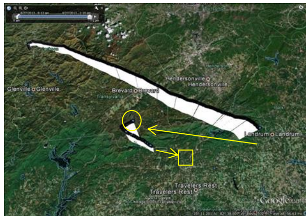
Figure 10: The Sparkfun data logger kml file of flight. The circle is Cat-5 maximum altitude. The arrows represent the direction the balloon was traveling during those gaps. The square represents the impact zone.
