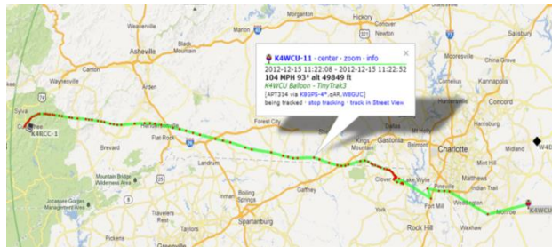
Figure 3: APRS flight path of Cat-4 from December 15, 2012. The beacon packets are transmitted every 60 seconds and show the balloon's flight path, altitude, heading, time, and mph it is horizontally traveling.
