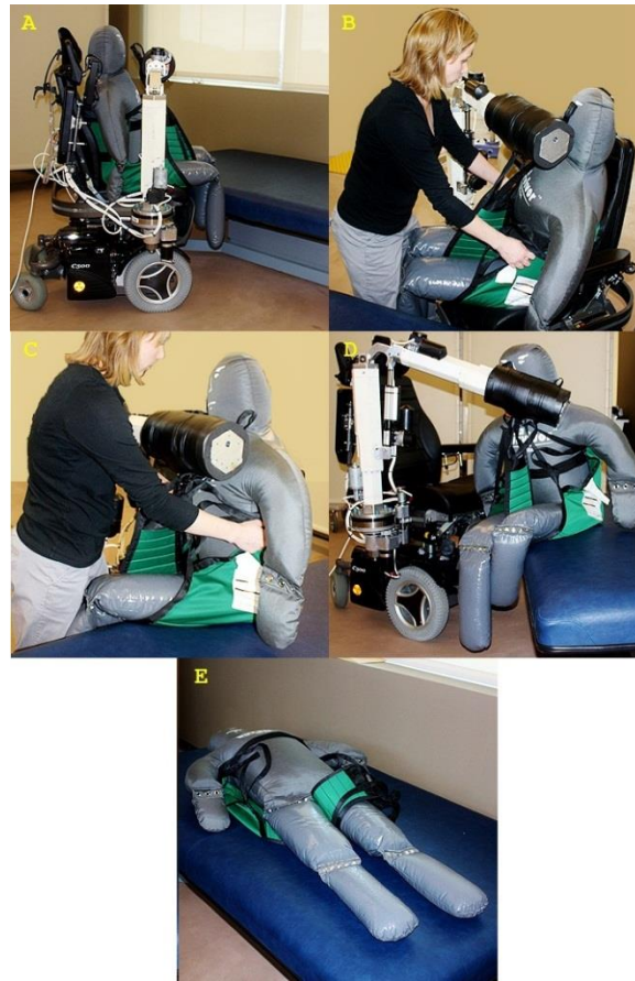
Figure 2. Steps A through E illustrate how the StrongArm attachment can be used to transfer a humanoid test dummy from a power chair to a bed.
