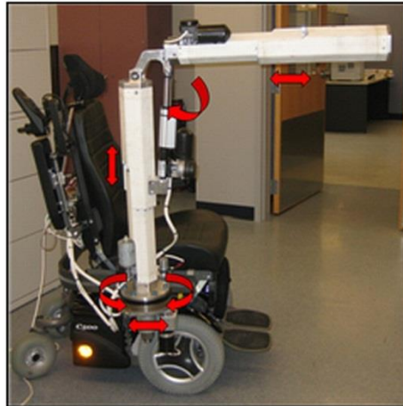
Figure 1. The five degrees of freedom of the robotic StrongArm are indicated with red arrows.
