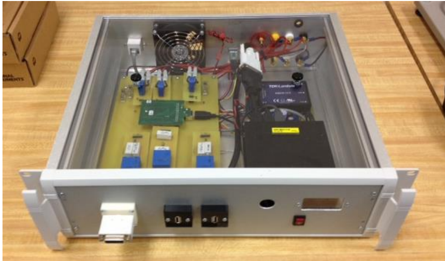
Figure 5. completed phasor measurement unit
