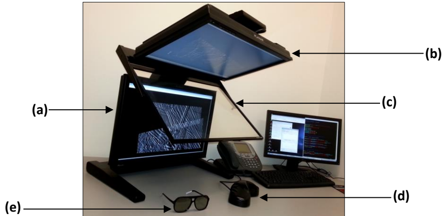
Figure 1. Workstation: (a), (b) stereoscopic displays (c) half mirror (d) 3D-topomouse (e) 3D passive glasses
