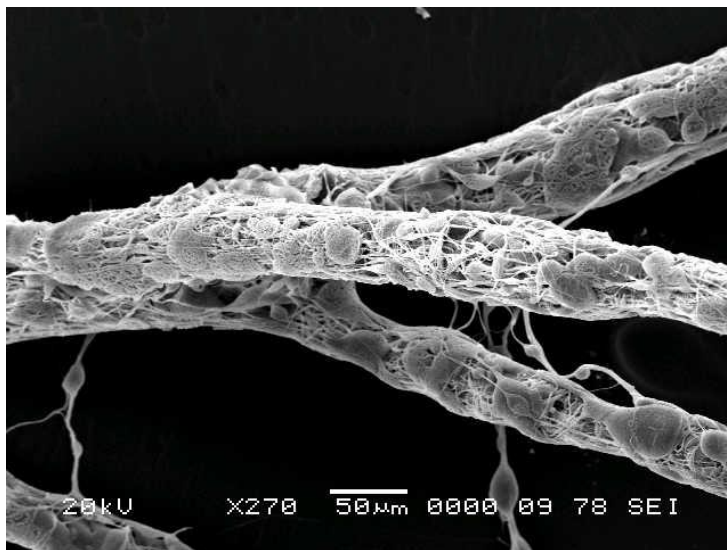
Figure2. SEM image of the ramification of the compound “root-like” fiber structure
