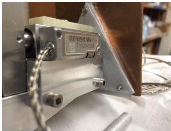
Figure 5. Encoder read-head mounted on the stepper motor.
