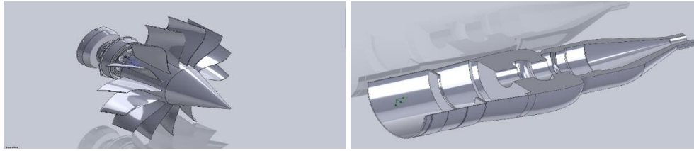
Figure 4. DGEN 380 prototype fan (left) and bi-sectional nacelle (right) in Solidworks
