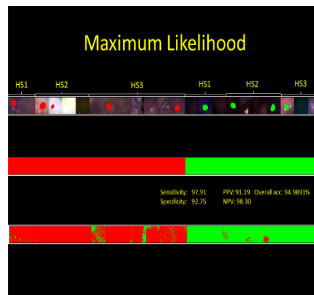
Figure 18: Maximum Likelihood. Classification of images were done using a supervised training algorithm called Maximum Likelihood. A confusion matrix was then used to determine sensitivity, specificity, and accuracy
