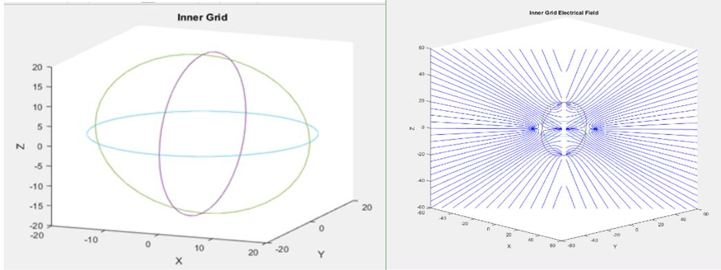
Figure 5: Inner Ring Geometry (Left), Inner Ring Electric Field Lines (Right)
