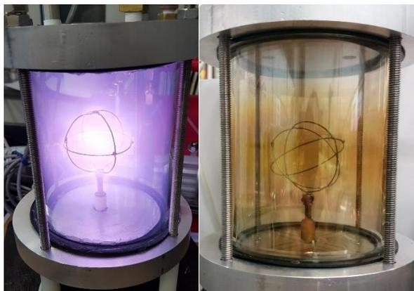
Figure 8. Final design, ‘star mode’ achieved (left) and particle deposition induced darkening phenomenon (right)
