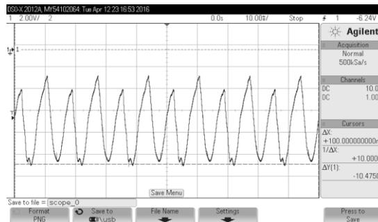
Figure 6. Oscilloscope reading of output voltage from rectifier
