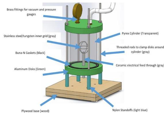
Figure 1. Complete fusor design detailing all mechanical components
