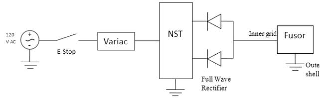
Figure 3. Circuit diagram for electrical subsystem
