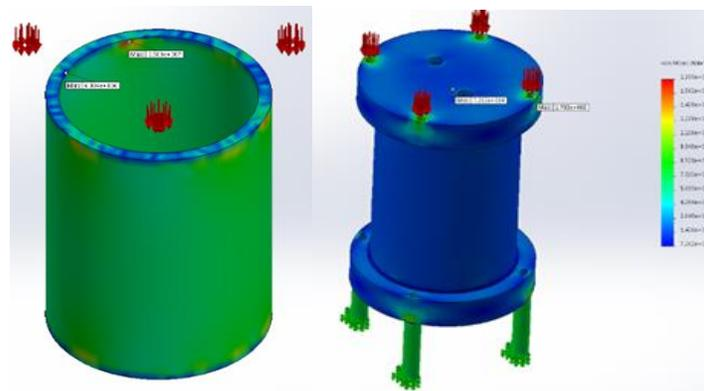
Figure 2. FEA analysis results showing tensile forces acting on the cylinder using Solidworks
