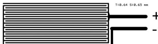
Figure 12. The shock capacitor design. Each arm of the comb has a width of 0.64 millimeters with a spacing of 0.65 millimeters between each arm.
