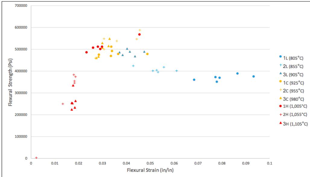
Figure 5. Flexural strength versus flexural strain of all samples
