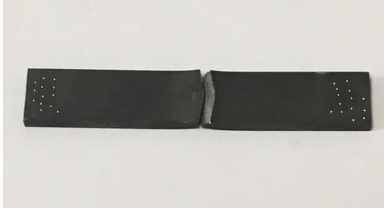
Figure 2. A2 steel sample with indenter marks from hardness test
