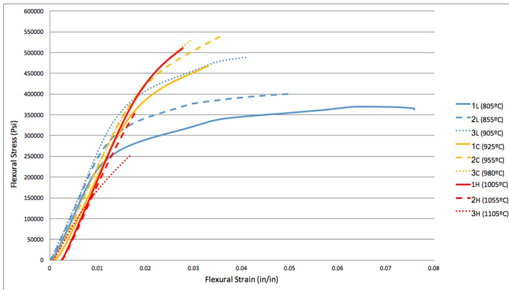
Figure 4. Flexural stress versus flexural strain
