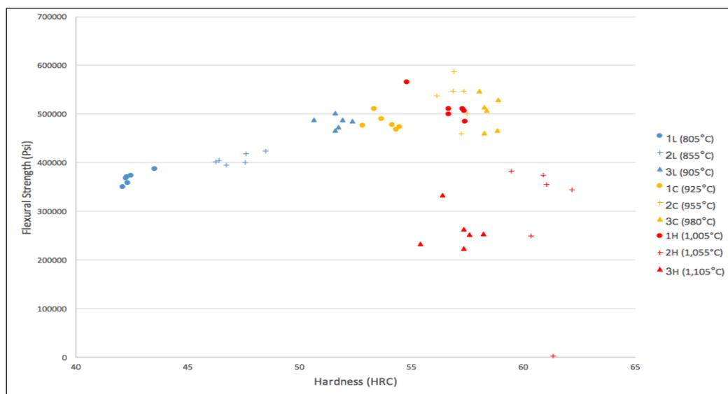
Figure 8. Flexural strength versus specimen hardness
