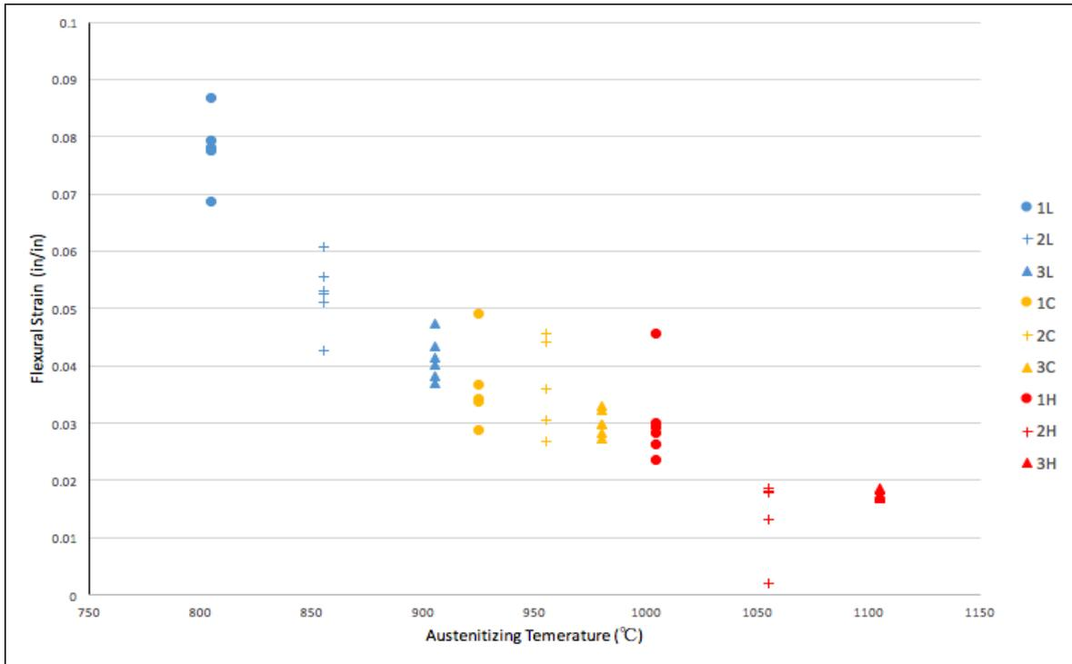
Figure 6. Flexural strain at breakage vs. austenizing temperature
