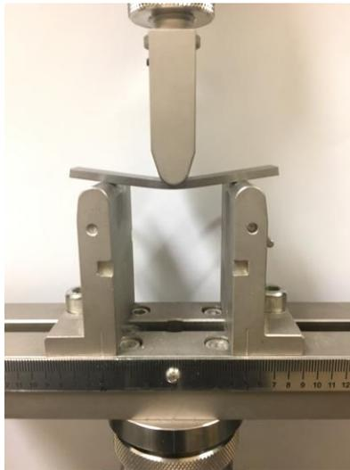
Figure 1. Flexural test
