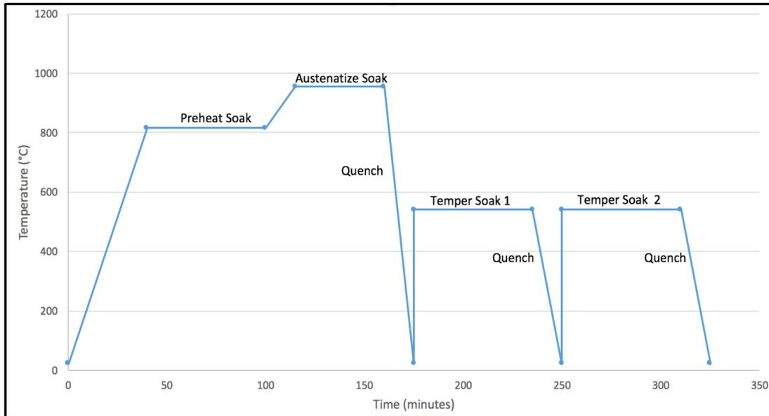
Figure 3. Phases of A2 steel heat treatment
