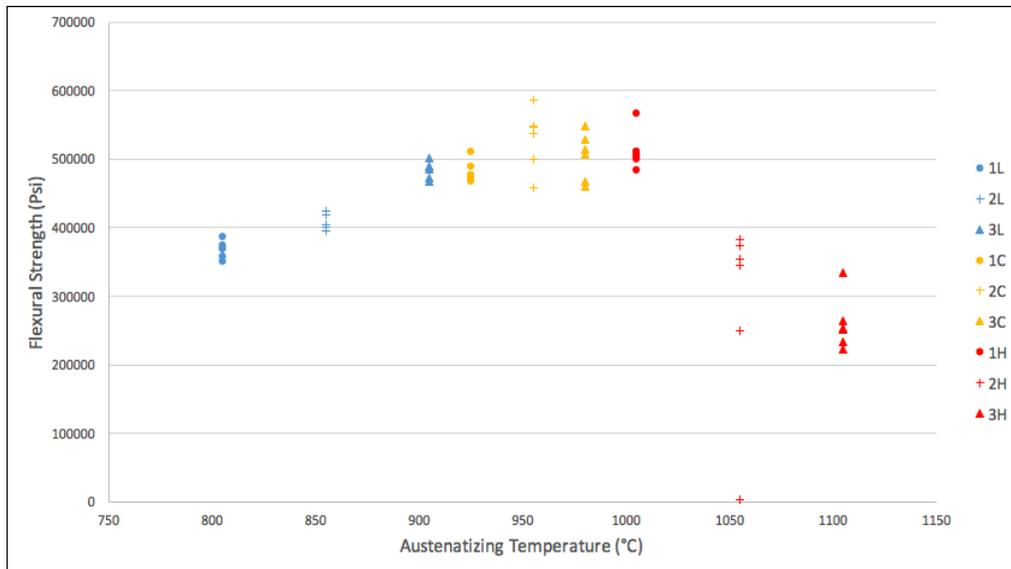
Figure 7. Flexural strength versus austenizing temperature
