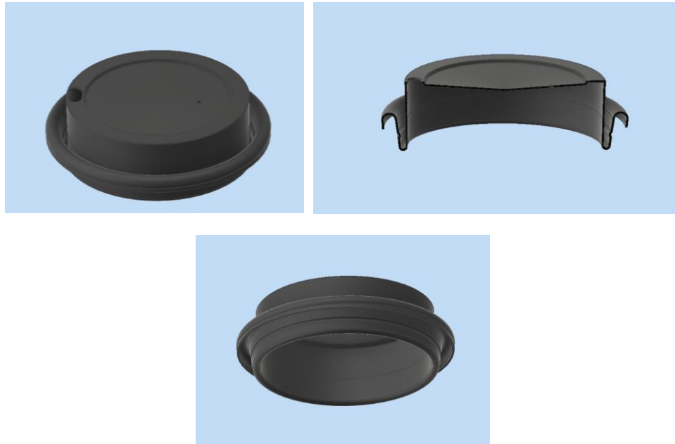
Figure 6. Coffee lid design 2, featuring the O-ring design
