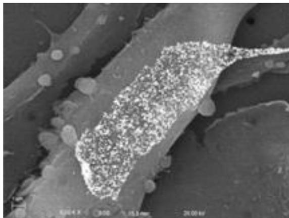
Figure 2. Transwell® with cells immediately fixed after gold aerosol particle deposition at the ALI
