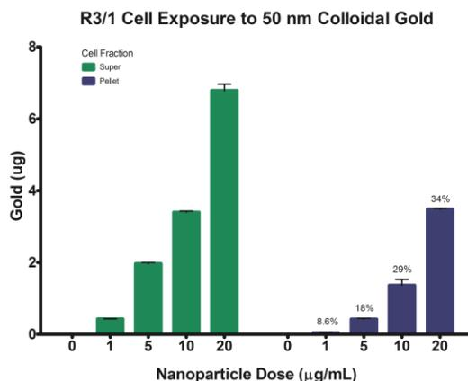
Figure 4. Measure of cell gold uptake following 4 h exposure n=3. Graphs show standard deviation. Percentages indicate the pellet fraction of the total dose delivered. Means ± SEM
