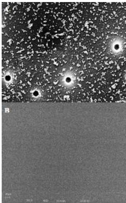
Figure 1. A. Transwell® containing media without cells. Gold NP deposition is shown at a magnification of 10,000 X, showing an ideal, even distribution of NPs. B. Transwell® containing media without cells, magnification of 200 X, showing an overall even distribution of gold
