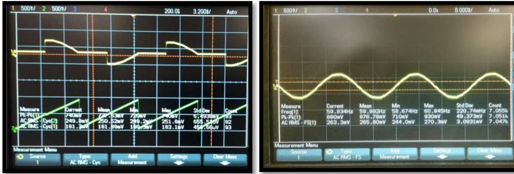
Figure 6. Phase Angle Control Circuit Set at 50% (left) and 100% (right)
