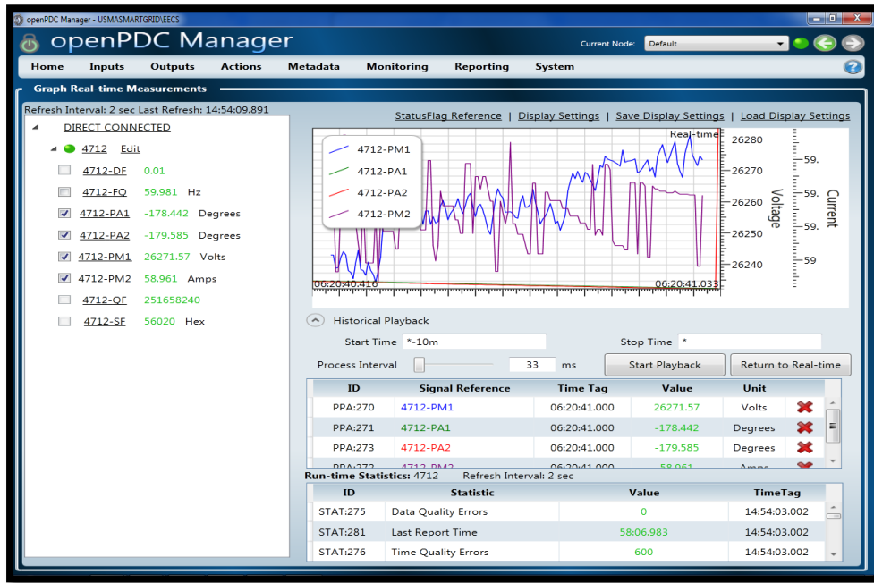
Figure 7. A screenshot of OpenPDC collecting data in real time
