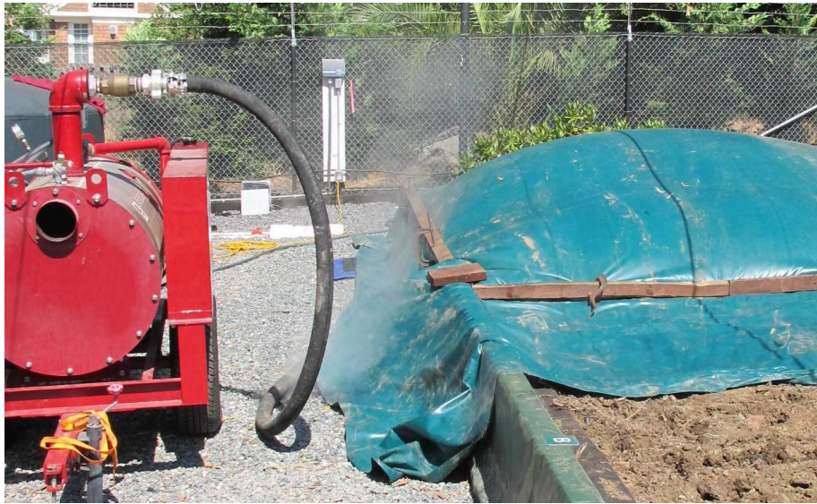
Figure1. Thermal treatment of Phytophthora samples at the NORS-DUC research nursery using a steaming unit SIOUX Steam-Flo SF-11.
