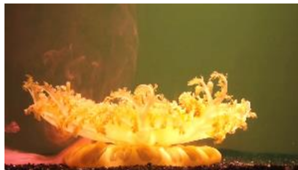
Figure 9. Dye propagation that shows mixing in the water column above the medusa due to its induced jet. This is the result of several bell pulsations without the presence of background flow.
