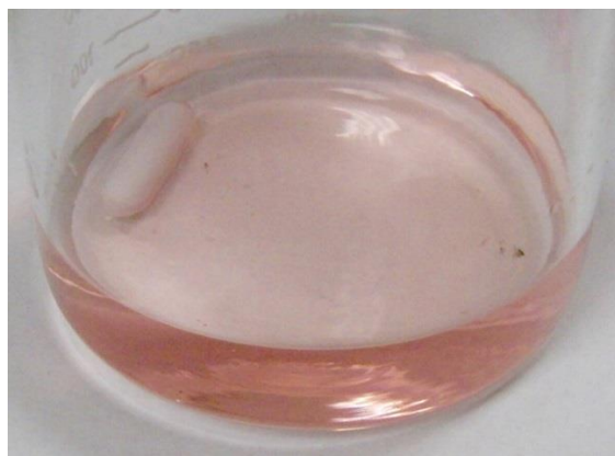
Figure 2.c Desired color at equivalence point (Carbonate).
