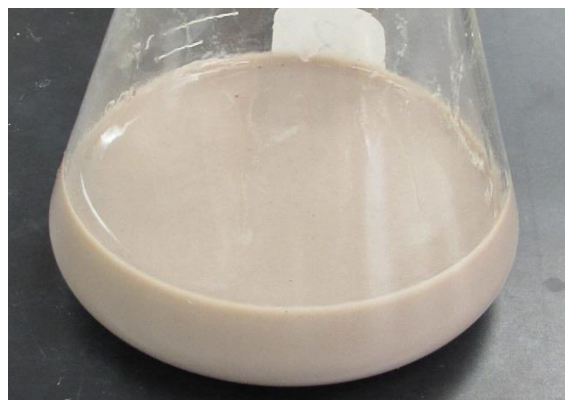
Figure 3.j QC analysis, after starch indicator with additional titrant added.
