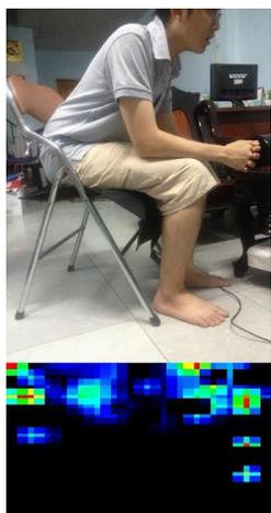
Figure 12. The pressure map showed a shift in pressure from lower area to the upper one when the user leans forward.
