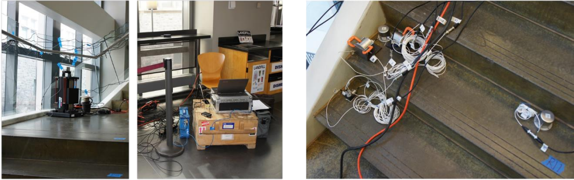
Figure 4. shaker, computer, and accelerometers used to test stair
