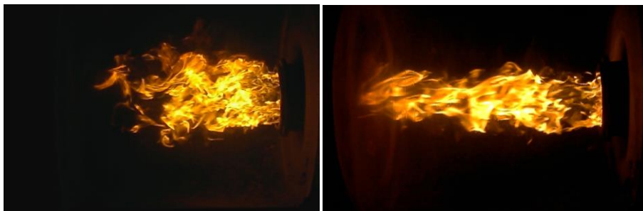
Image 7. Flame comparison in the quartz chamber between a 0% PS-Biodiesel (left) and a 0.5% PS-Biodiesel blend (right).
