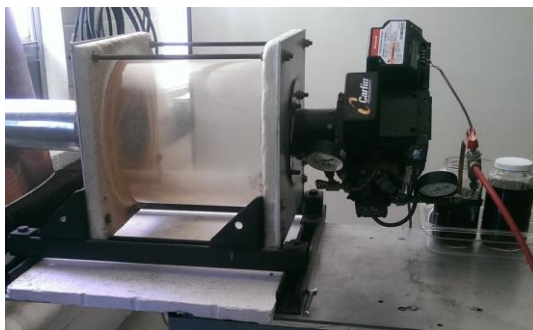
Image 3. Quartz chamber attachment to the Carlin fuel oil burner. The burner in this apparatus was set at 400 psi and the nozzle used was the 0.4 70-degree angle DoF nozzle.
