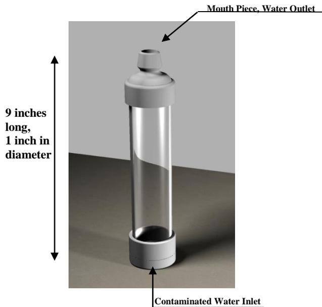
Image 1: Computer Design of Filter
