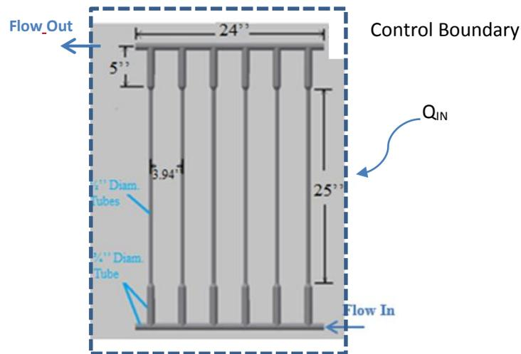
Figure 3: Control Boundary of Solar Collector
