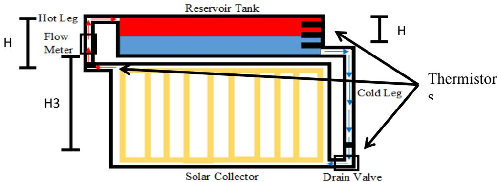
Figure 2: Horizontal Thermosiphon Schematic
