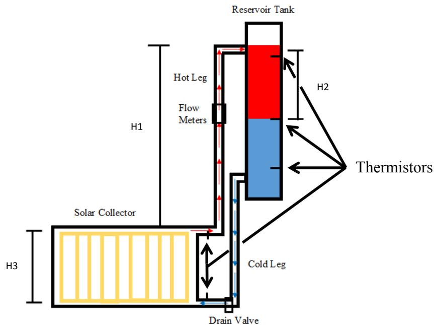
Figure 1: Vertical Thermosiphon Schematic
