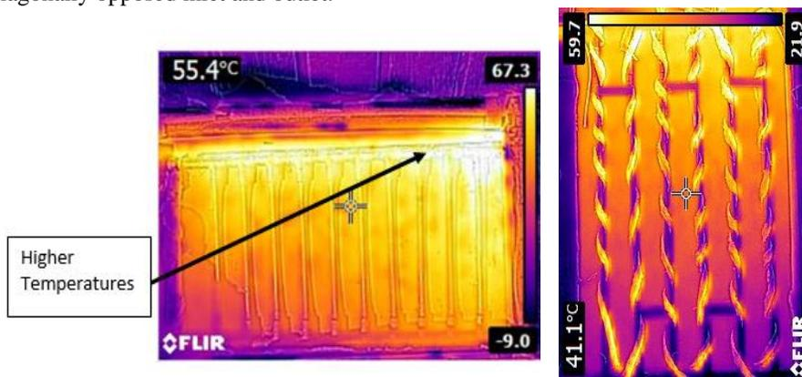
Figure 5: Infrared Display of Solar Collector
