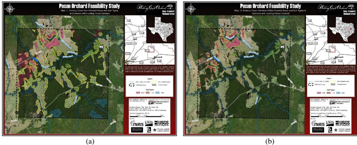
Figure 6. Hickory Creek non-forested areas and soil types in common with the existing orchard, and the results of executing the intersect operation.
