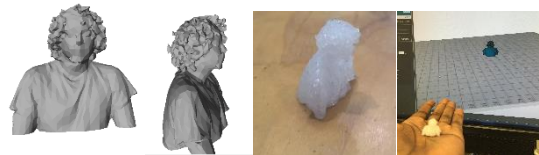
Figure 5 Notice the loss of detail in the smaller print compared to the 3D scan
