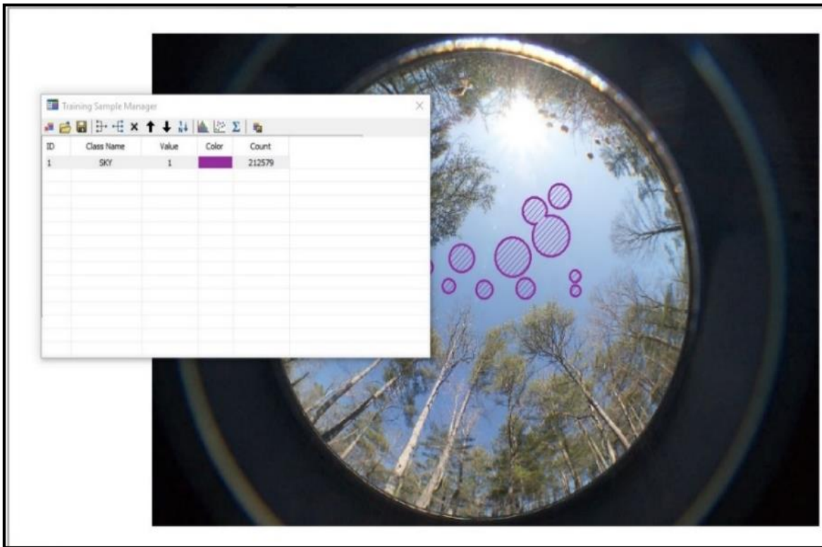
Figure 2: Selecting sample pixels of sky or open canopy for making a signature file in GIS Training sample manager window for a hemispherical photograph
