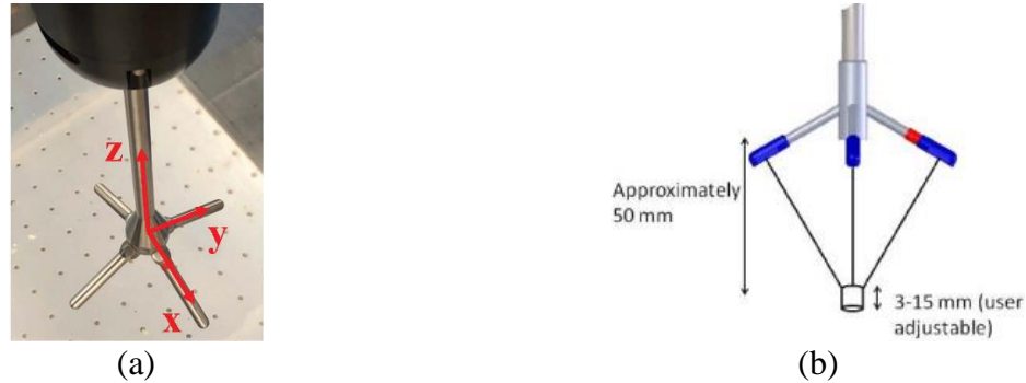
Figure 2. Nortek Vectrino’s transmitter and receivers (a) notation convention (b) sampling volume 8
