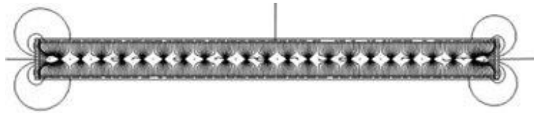
Figure 10. ComSol simulation of the electric field lines inside the entire chamber. The white regions are centered on the field shaping wires and the dark areas are where field lines converge on the anode wires. The isolation of anode wires is clear. Image courtesy of Dr. Kevin Stokes.
