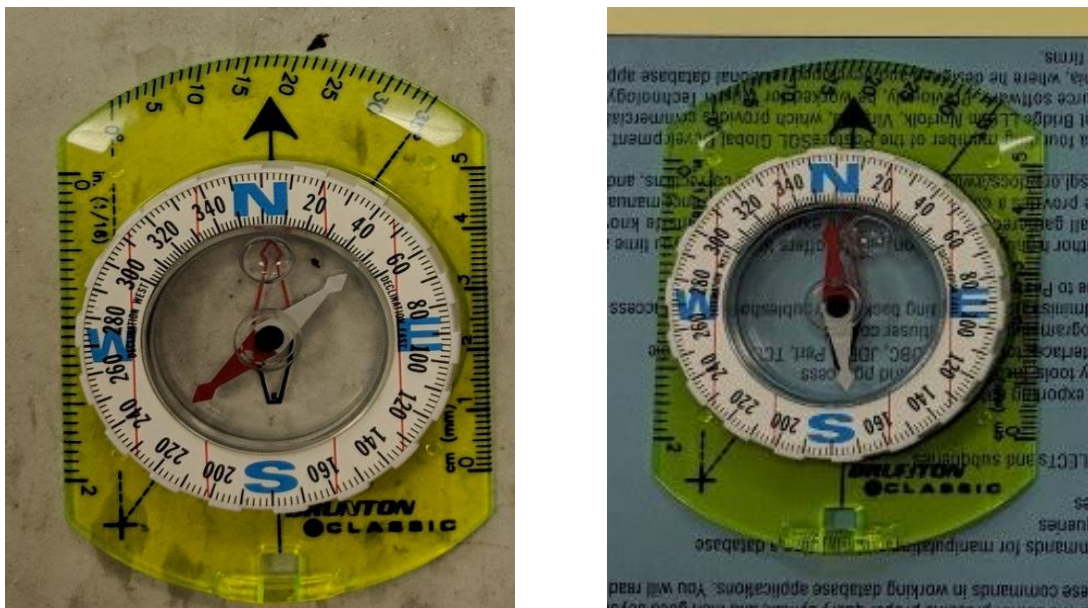
Figure 5. Compass placed on the same spot of the floor in the lab. Pictured right is the compass on a textbook. The left compass reads 230 degrees and the right compass reads 357 degrees.
