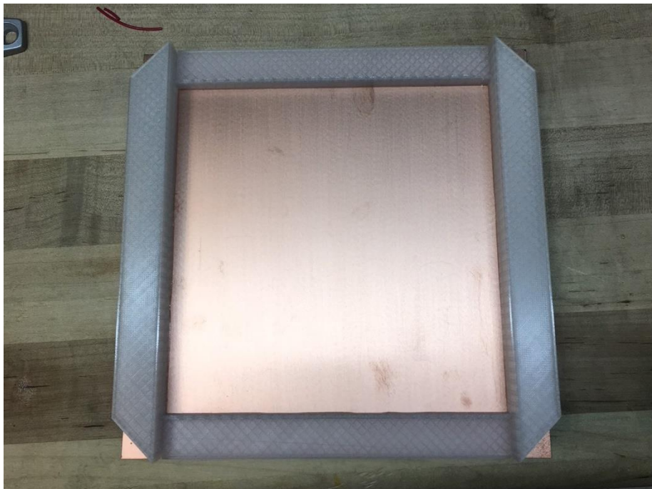
Figure 4. A 3D printed frame on top of a copper sheet. This prototype was from before O-rings were being used, so this one was intended to be sealed with glue.
