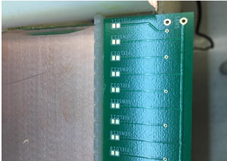
Figure 5. A close-up of one of the PCBs. The grooves on the frame can also be seen in this picture. The solder pads labeled “field” go to the ground wires, and those labeled “sense” go to the high voltage wires.
