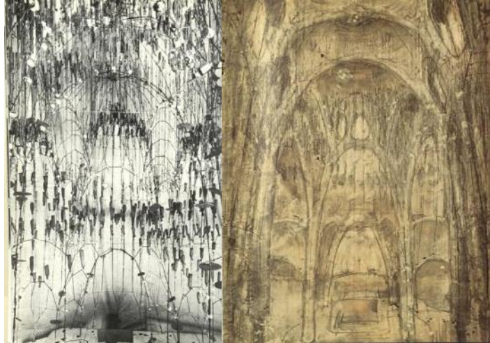
Figures 1 and 2. Funicular model showing structural design of Sagrada Familia by Gaudi [Image source: Descharnes, R., Pujols, R., Prévost, F., Pujols, Francesc, & Prévost, Clovis. Gaudí, the visionary. New York: Viking Press, 1982, Figs. on p.128 and 129]
