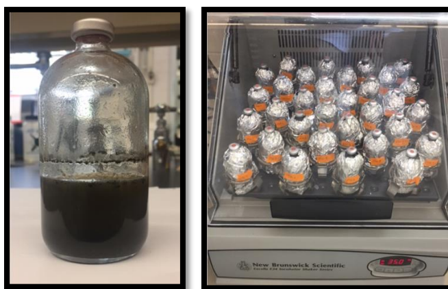
Figure 3: Loaded bioreactor (left) and shaker incubator (right)
