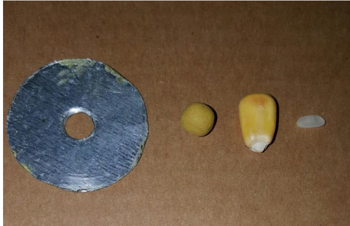
Figure 2: Sheet metal force disk, a single pea, kernel of corn, and grain of rice
