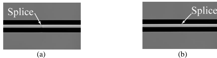
Figure 2: Images of two different fiber splices with (a) -0.11dB and (b) -0.02dB of measured loss, respectively.
