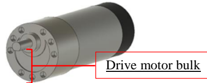
Figure 5: Fusion 360-generated 3D model of drive motor used in R-BEAR. The drive motors were installed with the bulk of the main body facing down towards the ground but must be rotated 180° to improve clearance.
