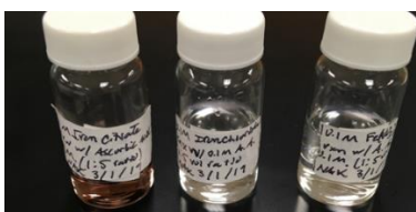
Figure 1: Reaction products of 0.1 M iron citrate (sample 5A), iron chloride (sample 5B), and iron nitrate (left to right) mixed in a 1:5 volume ratio with 0.1 M ascorbic acid. Sample 5A produced a colored solution and nanoparticles were visible after centrifuging the product.
