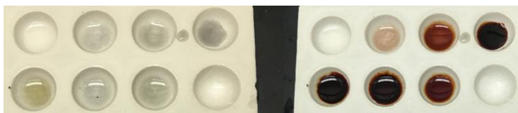
Figure 3: Samples before KSCN Addition (L) and after (R). Top left to right Acid Blank, Biochar Control, 5B, 3B. Bottom left to right 3C, 3A, 3E.
