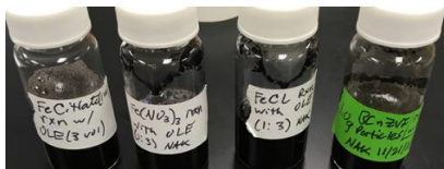
Figure 2: Reaction products of 0.1 M iron citrate, iron nitrate, and iron chloride (left to right) mixed in 1:3 volume ratio with OLE. The last vial is sample 4G contained 1 gram of the previously prepared biochar with adsorbed iron and was reacted with 10 mL OLE.
