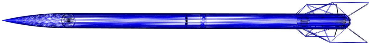
Figure 1. Industrial Trapezoidal Fin Configuration
