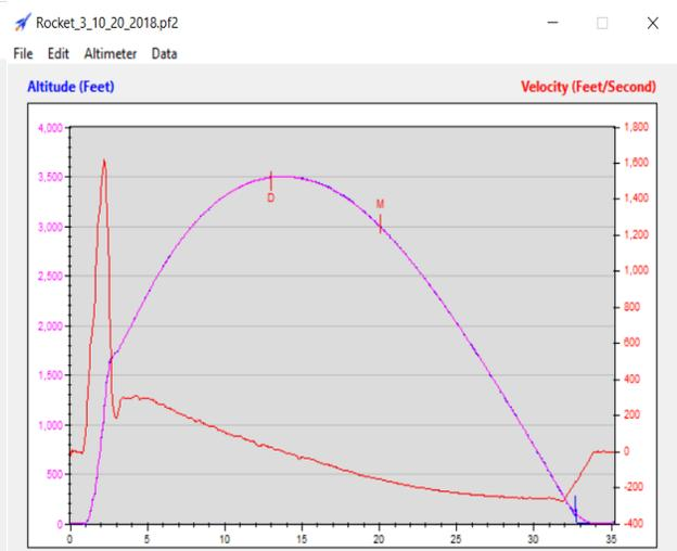
Figure 9. Flight Data from the Shark-Caved Fins Rocket
