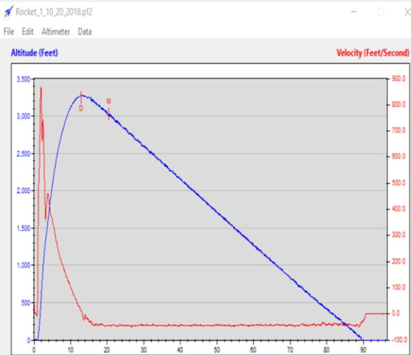
Figure 8. Flight Data from Trapezoidal Fin Rocket
