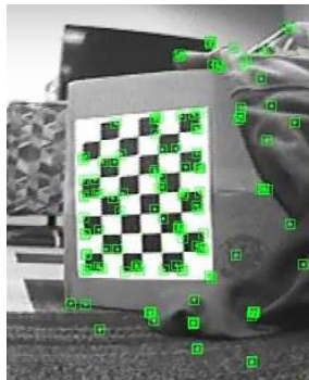
Figure 5. Output of SLAM from robotic snake stereo camera. Green rectangles indicate features within the environment recognized by SLAM.
