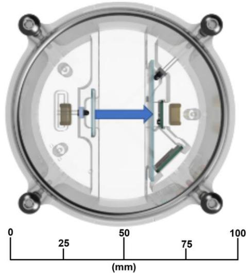
Figure 2. Light is emitted on one side of the channel, and read by the color sensor on the other. Both sensors are placed directly against clear acrylic windows to help prevent the reflection of light.
