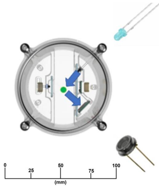
Figure 1. Integration of chlorophyll sensor into the detector. The green dot represents a water sample inside of a channel in the detector.
