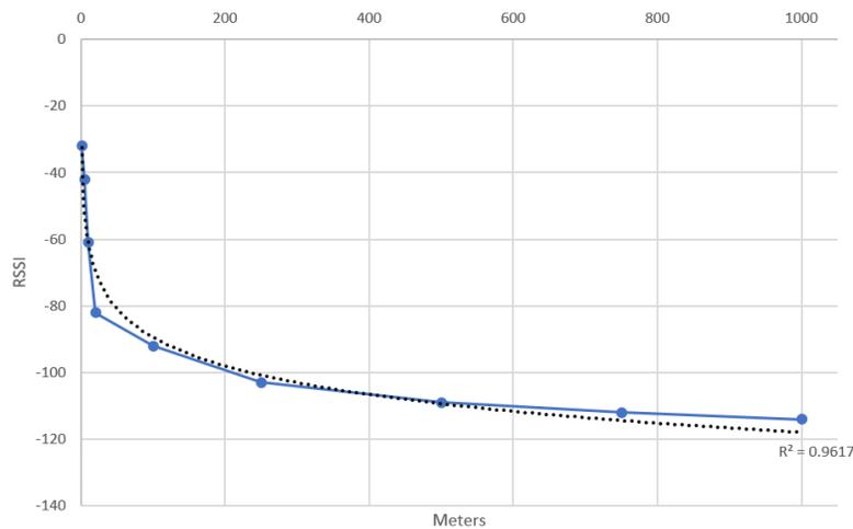
Figure 3. Received signal strength indication (RSSI) verses increasing distances.
