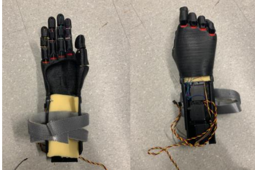
Figure 1. A 3D printed hand showing the palm of the hand and the back of the hand. This is a version of e-NABLE's open source Flexi Hand that we modified to accept servo motors.
