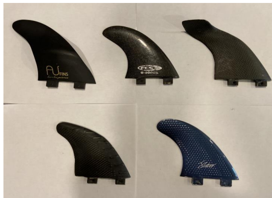
Figure 9: Fins from top left to bottom right: AU, FCS G-3000x (baseline), Phase II Winglet, Phase II Vortex Generator, Moonraker
