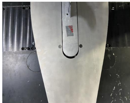
Figure 11: Potential spillage point between mounting block and panel.
