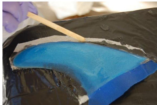
Figure 3: Coating Fiberglass on 3D Printed Fin which resembles the FCS baseline.
