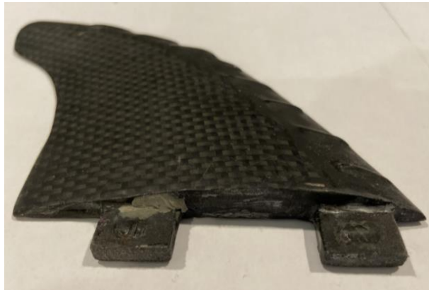
Figure 8: Image of inconsistencies on the Vortex Generator fin arising from the change in shape of the base of the fins at the fin tab attachment points.
